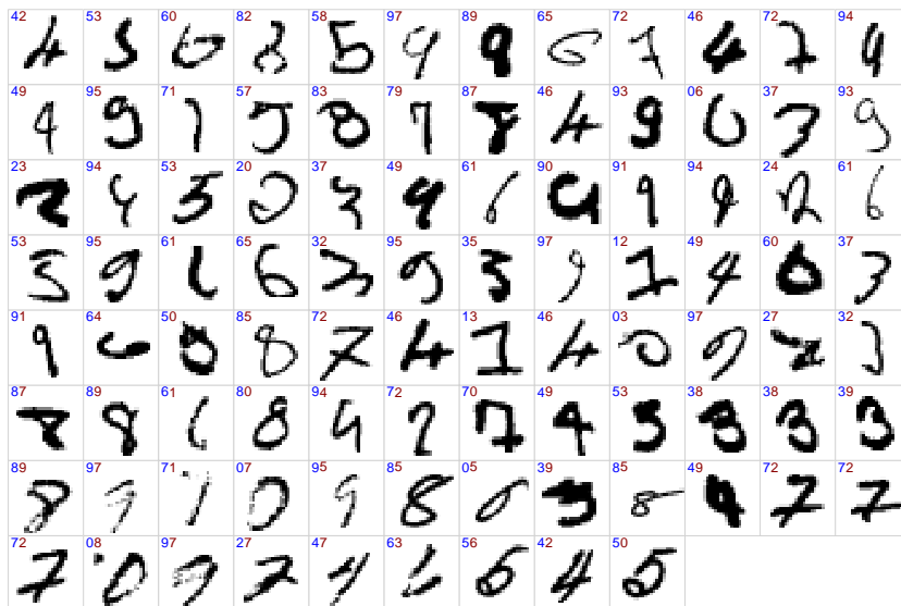
Figure 18.5 All 93 misclassified digits in the MNIST test set. The true digit class is labeled in blue, the predicted in red.
